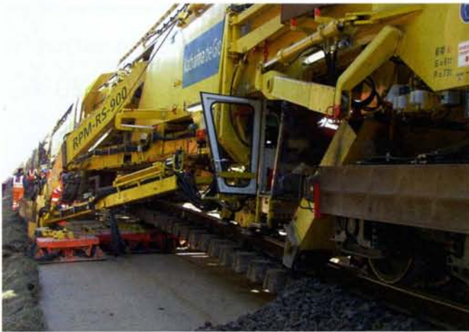
1 RPM-RS-900 track-laying machine: "Catherine the Great"
